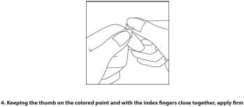
pressure on the colored point in the direction of the arrow to snap the ampule open. Step 4
